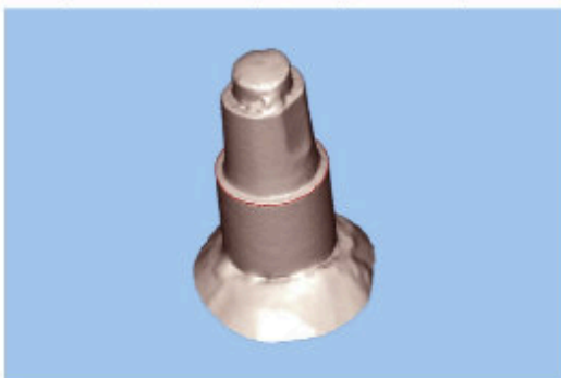
3 Computer-assisted design image obtained by scanning 4.1-mm abutment over 5.0-mm dental implant analog.
